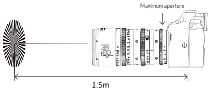
Set the object 1.5m away from the camera sensor plane, and adjust it to the center of the whole image.
